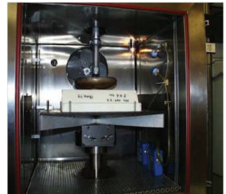
Figure 4: MDI-based polyurethane foam in the dynamic fatigue test chamber with air sampling pumps and sampling filters
