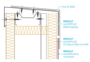
Fig. 2. gluing of parapets
