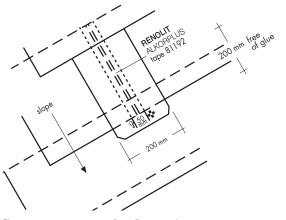
Fig.1. transverse seams of roofing membrane
